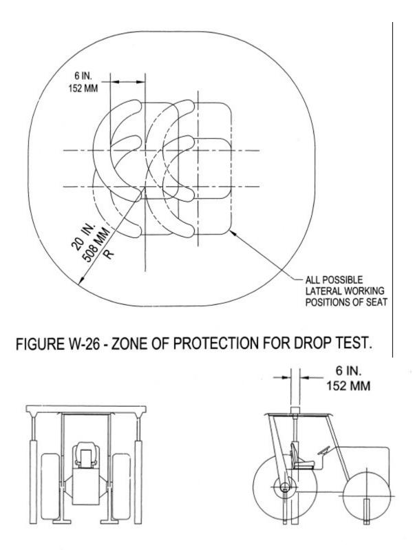
FIGURE W-27 - METHOD OF LOAD APPLICATION FOR CRUSH TEST.
