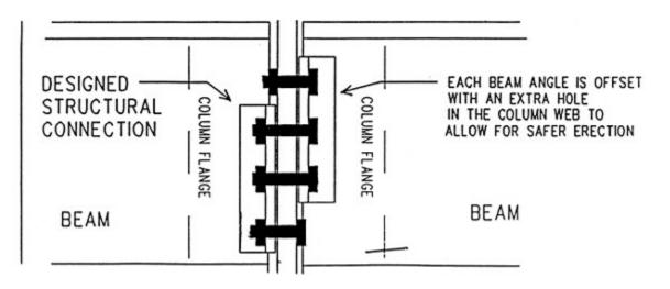
Staggered connections are connection material on a structural member in which all of the bolt holes in the common member web are not shared by the two incoming members in the final connection. The extra hole in the column web allows the erector to maintain at least a one
