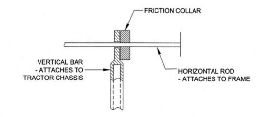
FIGURE W-18 - METHOD OF MEASURING INSTANTANEOUS DEFLECTION.
