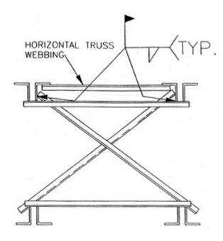
JOISTS PAIR BRIDGING TERMINUS POINT W/HORIZ. TRUSS
